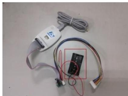
DC 3V (AA size Battery x 2) for Console PCB
