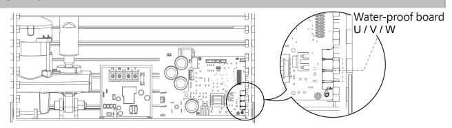
Pull out the motor wires (U.V.W)
