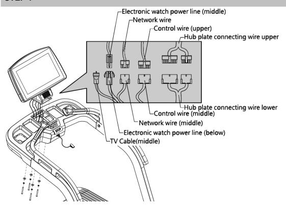
Take off the screw and washer in the computer console and water bottle shelf, and then plug out the wire to take off the computer console.
