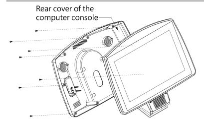
Loosen the fixing screws of the computer console, carry up the rear cover of the computer console and then take up the rear cover of the computer console.
