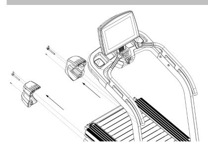
Loosen the fixing screws for the left and ring front adjusting caps, and take off the adjusting caps.
