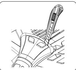
Embed the knife into the space between the control box and handrail to turn up the gel key to change the control box and gel key.
