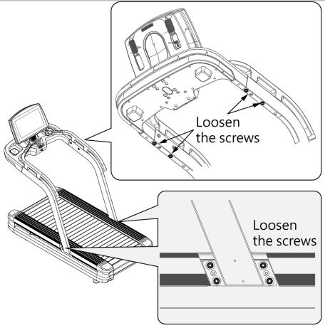
Loosen the screws on the image above.
