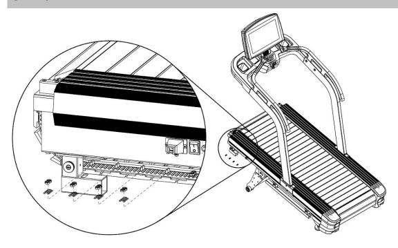
Loosen nylon nuts and padding plated at the left and right sides in the running board which should be changed, according to the image.
